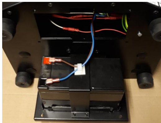
Figure 4 Battery module with battery secured and connected
